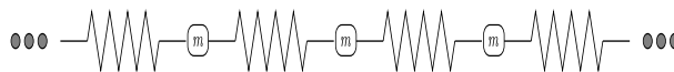
Fig. 2. Multiple springs and masses. In this setup, displacing one of the elemental masses from its rest position, besides setting that mass in motion as in the simpler model of Fig. 1, also has the effect of inducing motion on neighboring masses. Therefore, the oscillations of individual masses are clearly not independent, but coupled through the springs that bind them.
