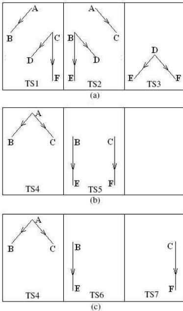
Fig. 3. Illustration of optimal schedules for coding (a) and routing (b). An alternative schedule for routing is given in (c). Each box shows a set of wireless links that can be simultaneously activated, termed a transmit scenario (TS).
