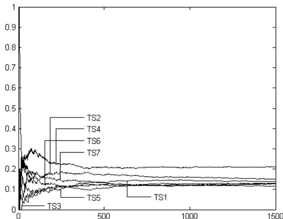
Fig. 6. The proportion of different transmit scenarios used by the routing algorithm for  $\text{snr} = 10$  (10dB),  $a = a_1 = a_2 = \sqrt{2}/2$ ,  $k = 2$ ,  $\mu = 1.5$ , transmission rate = 1.3.
