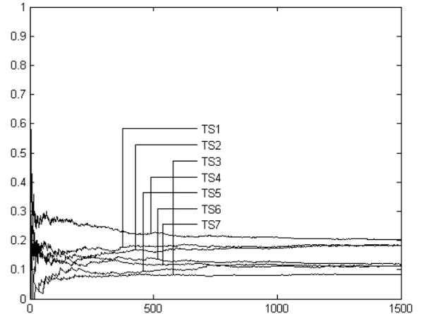
Fig. 4. The proportion of different transmit scenarios used by the network coding algorithm for  $\text{snr} = 10$  (10dB),  $a_1 = a_2 = a = \sqrt{2}/2$ ,  $k = 2$ ,  $\mu = 1.5$ , transmission rate = 1.4.
