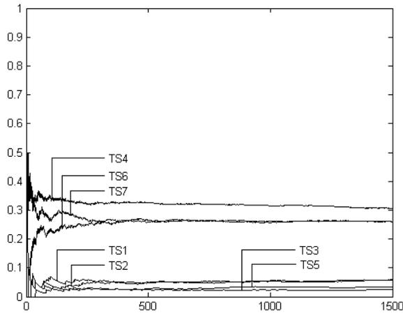
Fig. 5. The proportion of different transmit scenarios used by the network coding algorithm for  $\text{snr} = 100$  (20dB),  $a_1 = a_2 = a = \sqrt{2}/2$ ,  $k = 2$ ,  $\mu = 1.5$ , transmission rate = 2.3.
