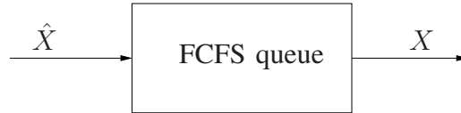
Fig. 1. The Diagram of interpreting \mathcal{X} as the output of a FCFS queueing system with \hat{\mathcal{X}} as the input. The point process \mathcal{S} is defined by treating inter-arrival time S_i as the i th service time.
