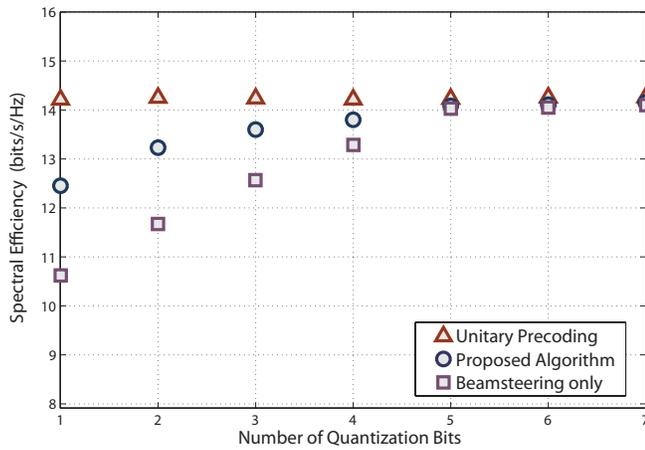
Fig. 4. Spectral efficiency as a function of phase quantization bits in a hybrid system with only quantized analog phase control. Results are reported for a  $40 \times 10$  mmWave system at an SNR of 0dB.
