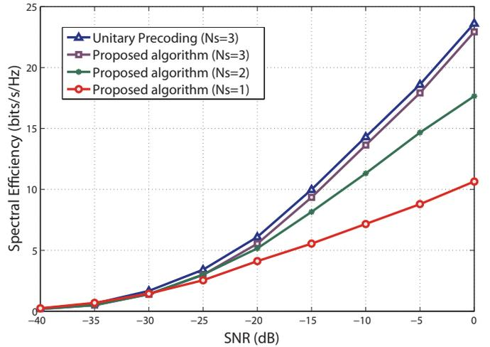
Fig. 3. Spectral efficiencies achieved by the proposed hybrid analog-digital precoding algorithm in a  $200 \times 100$  mmWave system with 3 RF chains at both the BS and MS. The figure indicates that the proposed strategy can achieve near-optimal performance despite its low hardware complexity and reliance on partial channel knowledge.
